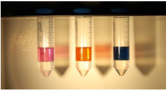
Metal ion extraction from water by hydrophobic DES (Deep Eutectic Solvents),
